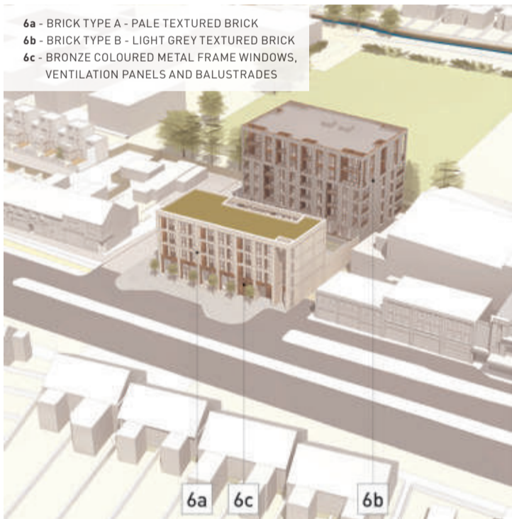
AERIAL OVERVIEW SHOWING MATERIALS FOR PHASE 1
